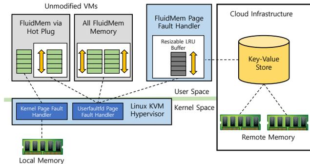
Figure 1: FluidMem Architecture
