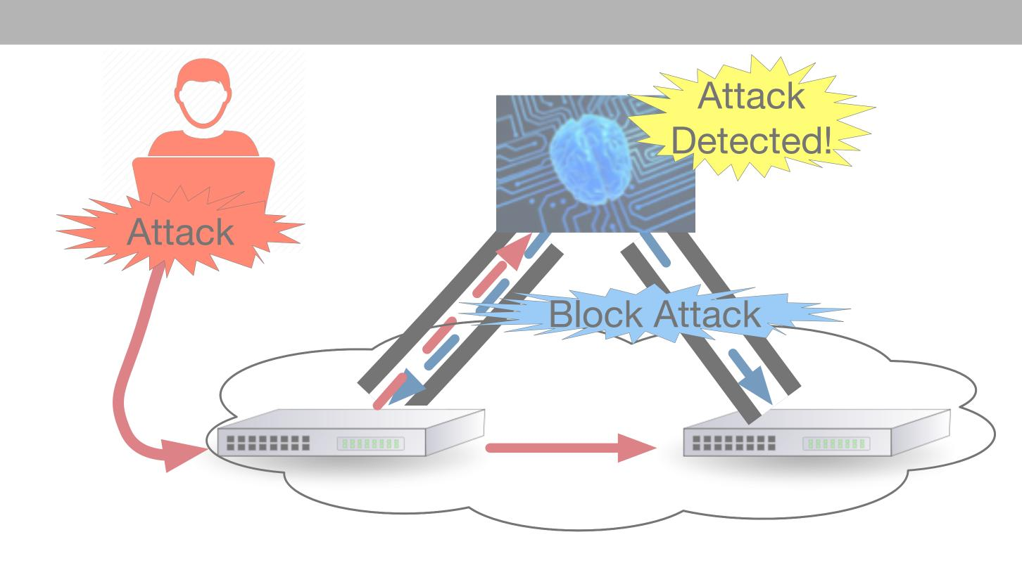
OpenFlow security applications can program switches but must do advanced processing and flow set up at the centralized OpenFlow controller, which limits performance and scalability.
