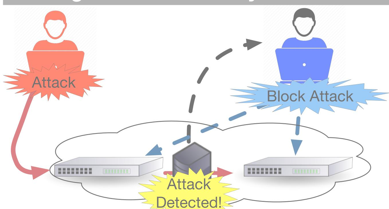
Traditional network security applications are deployed onto middlebox servers and have limited control over traffic or the network.
