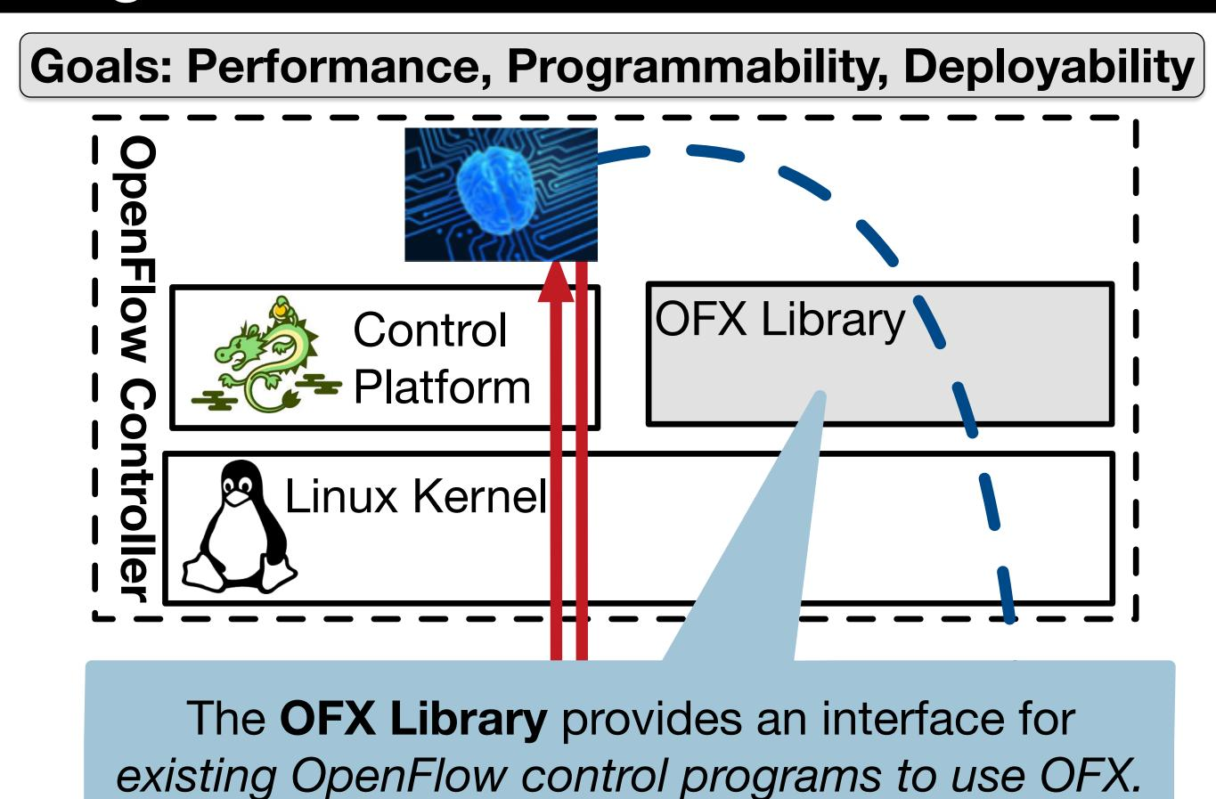
**OFX Agents** run the **OFX Extension Modules** Extension Modules on implement new switch unmodified OpenFlow functionality in C and Python. Switches.
