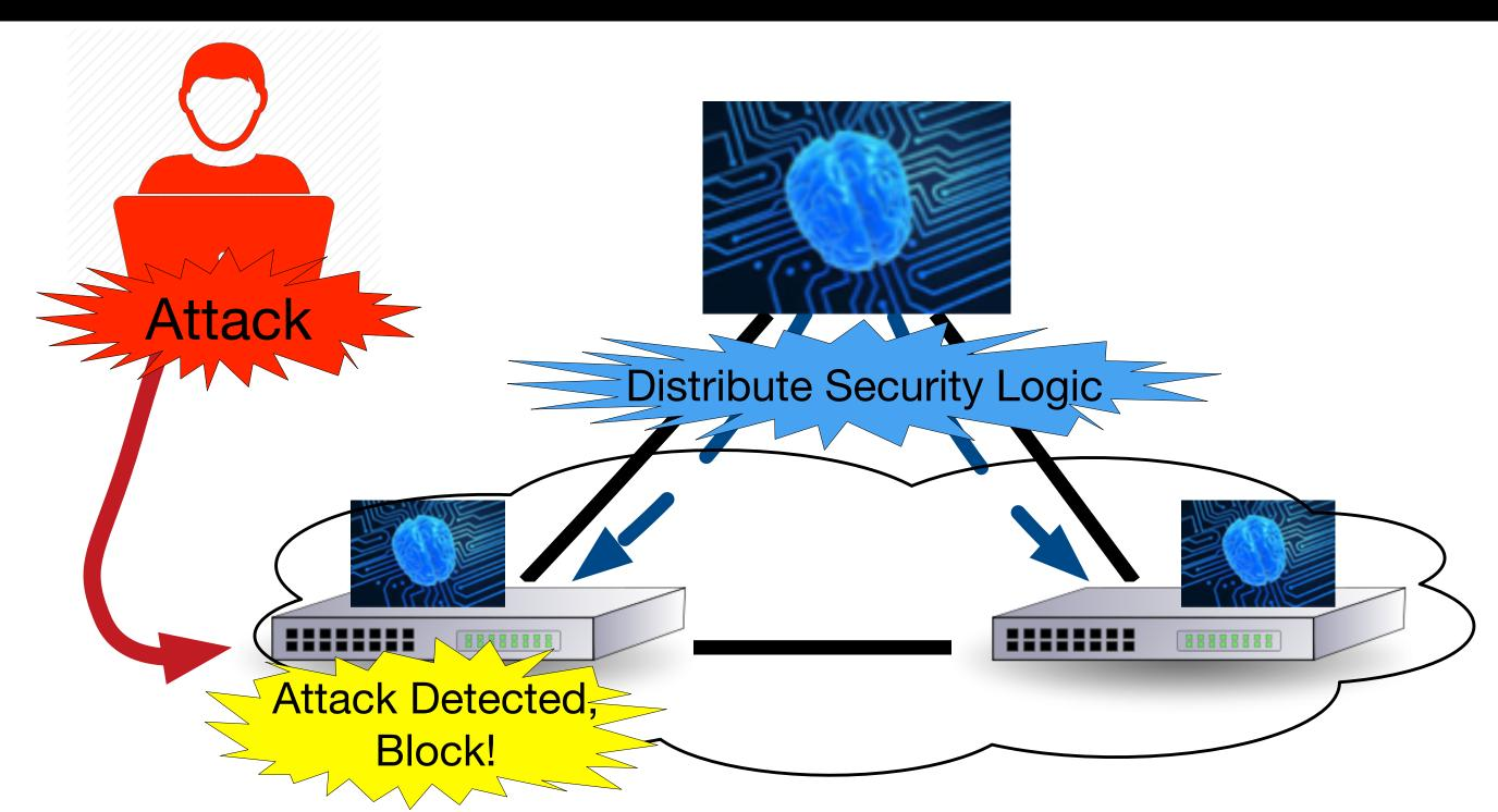
OFX improves OpenFlow security application performance and scalability by allowing them to install custom software modules to process packets and set up flows at the switch.
