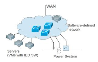
Fig. 3. Future substation with virtualized IEDs.
