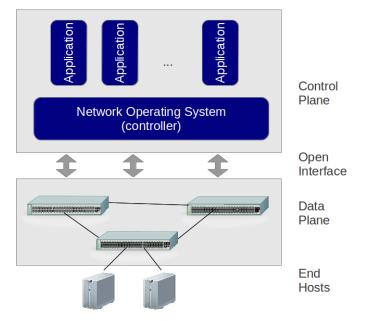
Fig. 1. Overview of SDN architecture
