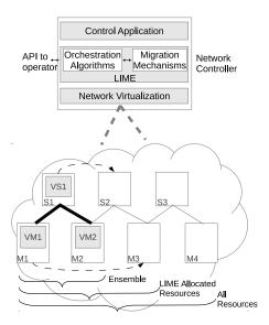
Figure 2: LIME architecture with example. The virtual network consists of two VMs and a virtual switch which are presently mapped to physical devices within a larger infrastructure. To migrate one VM and one virtual switch to different physical devices, LIME works with the virtualization layer to extend the resources allocated to the virtual network during the migration.
