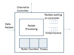
Figure 1: SDN switch state.
